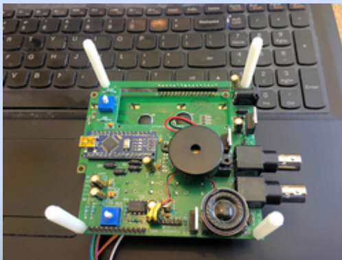
The ventilator controller circuit board, designed by Michael Stapleton, WD4LHT. [Courtesy of Gordon Gibby, KX4Z]
