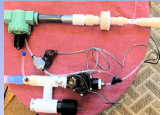
Airway components of the emergency ventilator. [Photo courtesy of Gordon Gibby, KX4Z]
