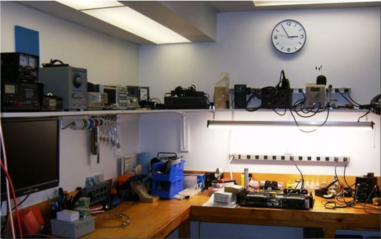
Basement workshop, obviously not cleaned up for the photo, overall view. The 224.180 repeater is on the bench for installation of the repeater controller / CW ID unit.
